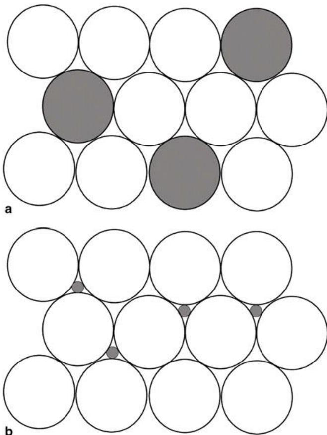
**Figure 3.** a. Substitutional crystalline solid solution
