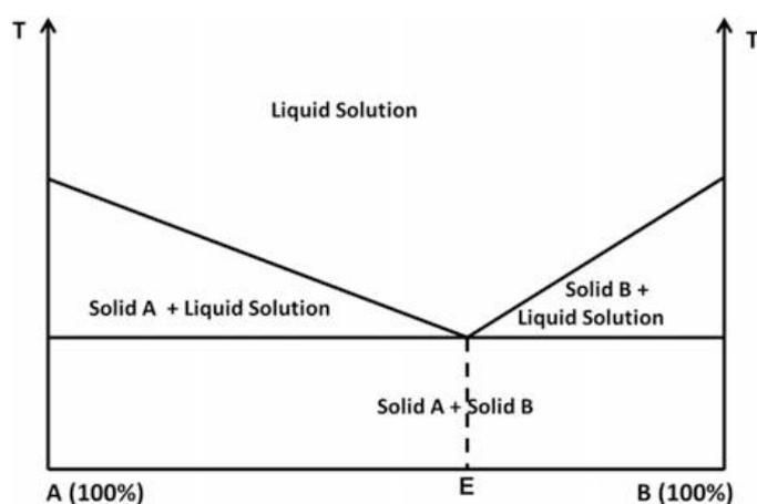
**Figure 1.** Phase diagram of a simple eutectic system
