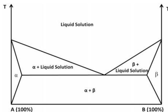
**Figure 2.** Phase diagram of a discontinuous solid solution
